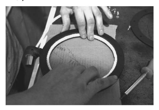
2: PLACE THE NEW GLASS ON TOP OF THE NEW ROPE, ALIGN EVENLY AND BED IT IN BY PRESSING IT FIRMLY AROUND THE EDGES.
