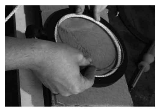
3: PLACE THE DOOR FRONT IN POSITION AND INSERT ONLY THE TOP AND BOTTOM BOLTS. ONLY SCREW THEM IN A COUPLE OF THREADS – JUST ENOUGH THAT THEY WON'T PULL OUT WHEN YOU ARE FITTING THE SECOND ROPE
