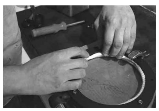
9: WHEN THE ROPE IS PUSHED IN ALL THE WAY AROUND, ANY BITS WHICH HAVE BEEN PUSHED TOO FAR IN, CAN BE GENTLY PUSHED BACK INTO PLACE WITH A BLUNT FLAT OBJECT. I WOULD RECOMMEND A BUTTER KNIFE FOR EXAMPLE.
