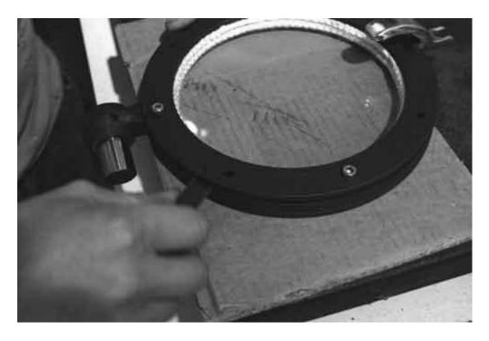
10: FINALLY, TIGHTEN UP THE 3 BOLTS A FEW MORE TURNS AND THEN REPLACE THE OTHER 4 BOLTS AND TIGHTEN THEM ALL A FEW TURNS AT A TIME TILL THE ARE ALL HAND TIGHT.
